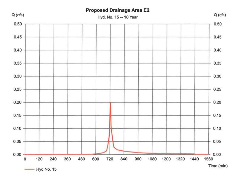
Hydraflow Hydrographs by Intelisolve v9.23
