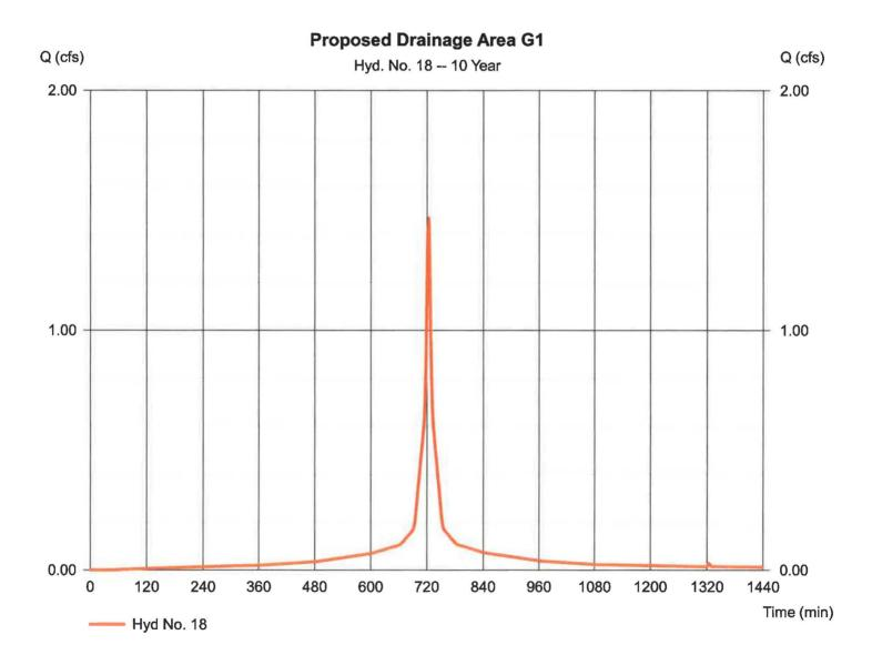
Hydraflow Hydrographs by Intelisolve v9.23
