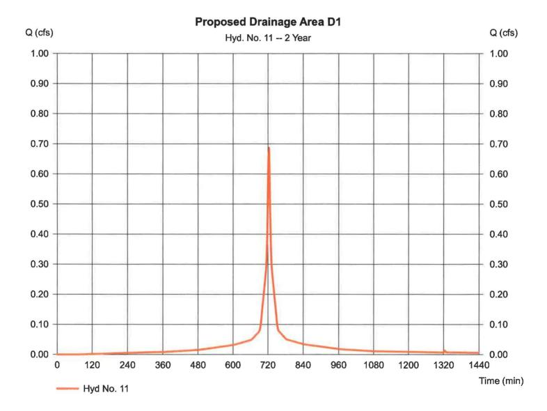
Hydraflow Hydrographs by Intelisolve v9.23
