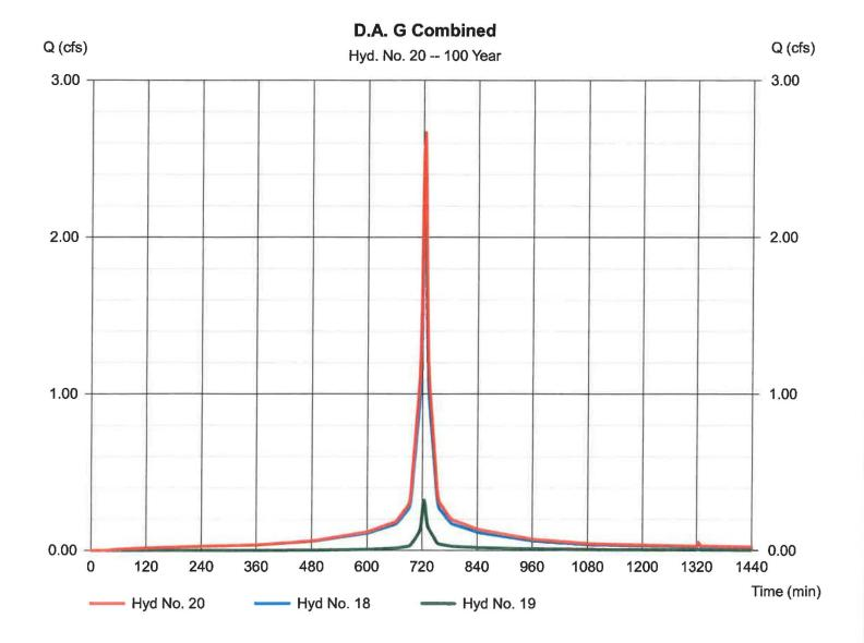
Hydraflow Hydrographs by Intelisolve v9.23
