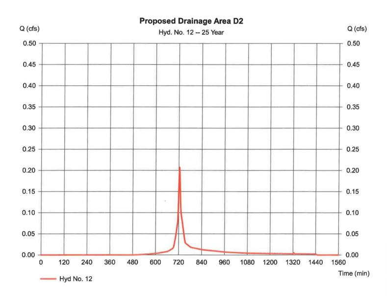
Hydraflow Hydrographs by Intelisolve v9.23
