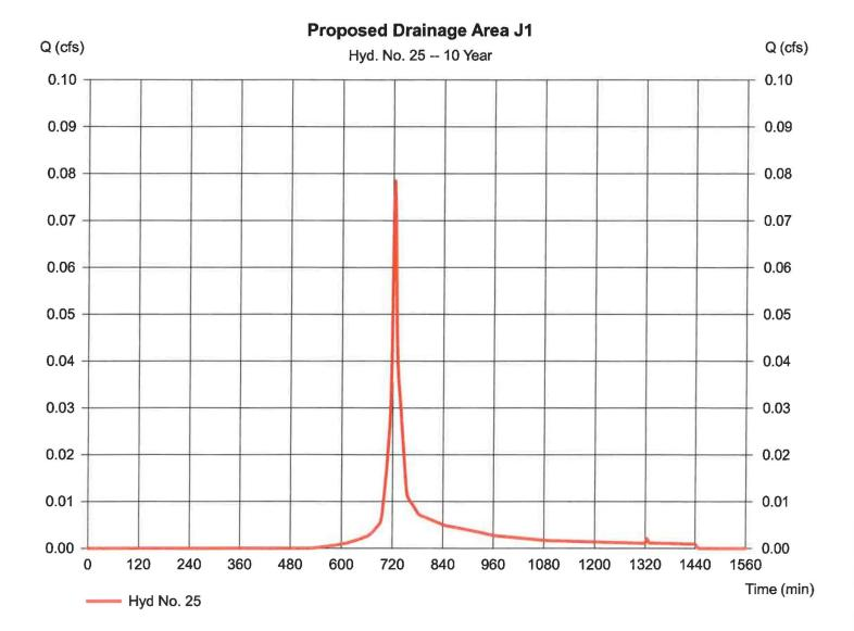
Hydraflow Hydrographs by Intelisolve v9.23
