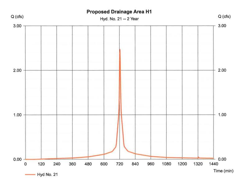
Hydraflow Hydrographs by Intelisolve v9.23
